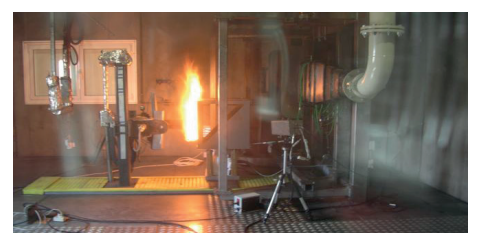
Fire testing on CFRP panel
