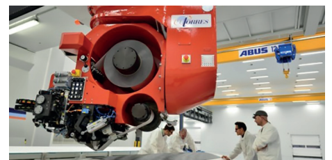
ATL ply deposition prior to SQRTM curing
